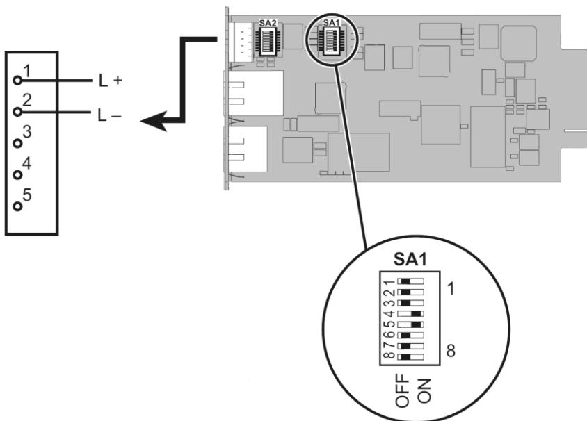
Set the SA1 switches to select the **two wires** configuration with **termination**:
