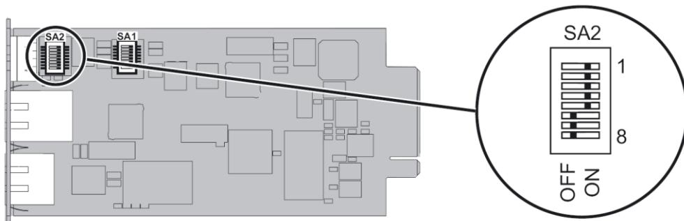
Set the SA1 switches to select the **four wires** configuration with **no termination**:
