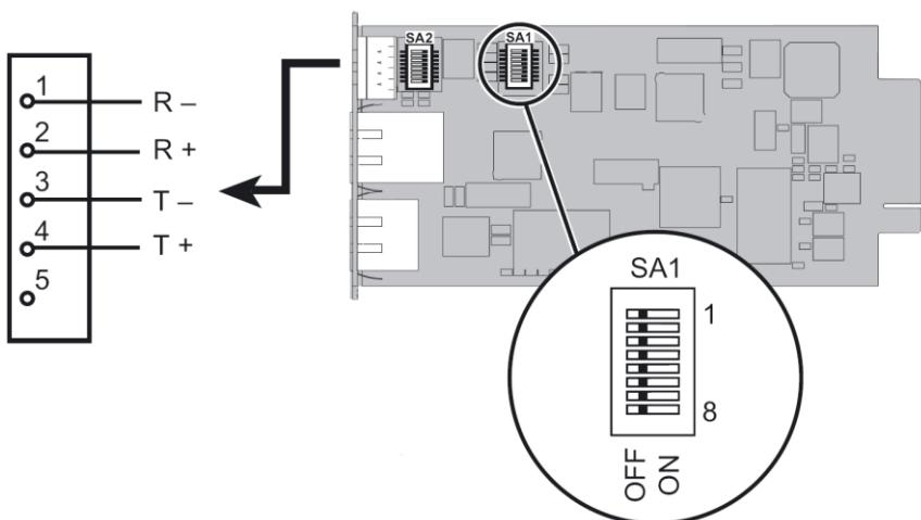
Set the SA1 switches to select the **four wires** configuration with **termination**:
